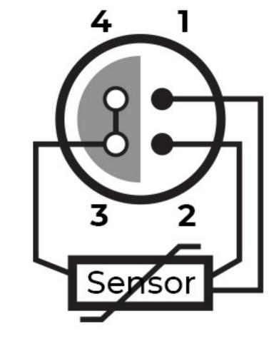
Shield electrically connected with tube & housing.
